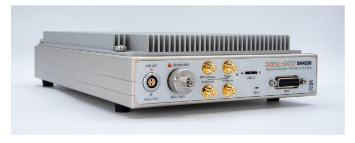
The SM435B is a high-performance spectrum analyzer and monitoring receiver. Tuning from 100 kHz to 43.5GHz, the analyzer has 160 MHz of instantaneous bandwidth (IBW), 110 dB of dynamic range, 1THz/sec sweep speed at 30kHz RBW (using Nuttall windowing), and ultra-low phase noise to rival even the most expensive spectrum analyzers on the market.
